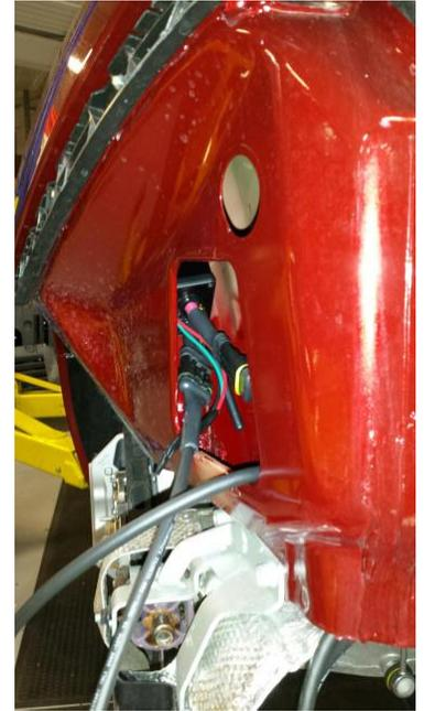
A more secure location is to route the cables inside the vehicle's luggage compartment and install the controller in the luggage compartment. This will require finding a suitable hole where you can pass the cable through into the luggage compartment. If a suitable hole cannot be found, a hole will need to be cut.
