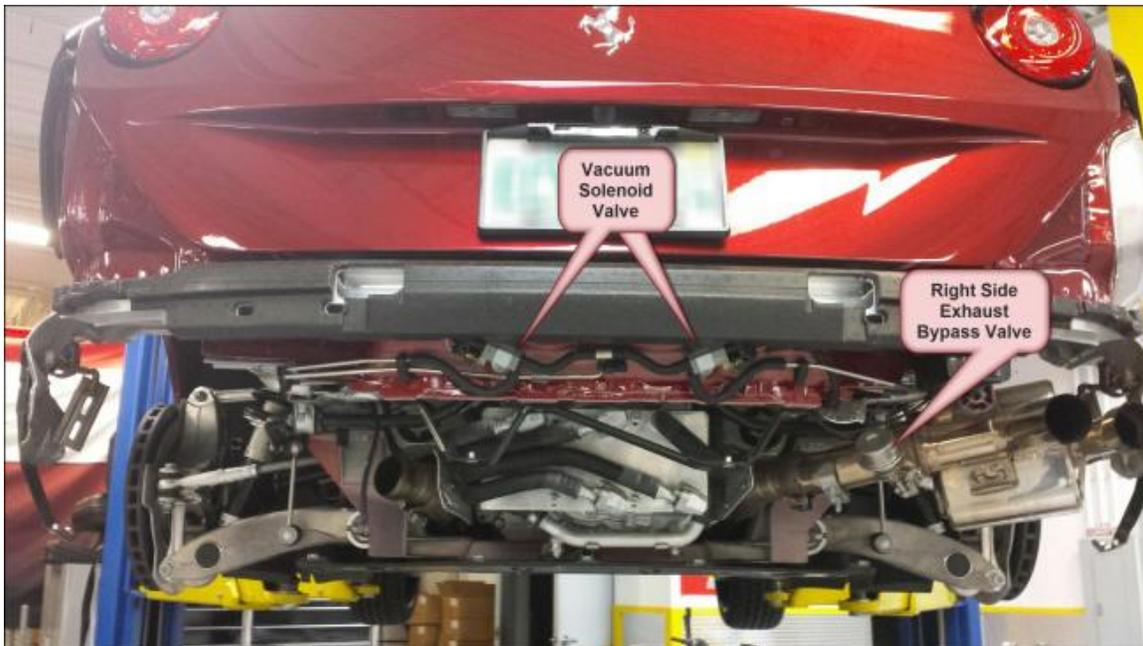
*Note: The photos show the rear bumper removed. Before actually removing the rear bumper, check to see if you can gain access to the vacuum solenoid valves by removing the rear diffuser only. Some have indicated that, although a tight squeeze, a person with small hands may be able to access the valves.*
