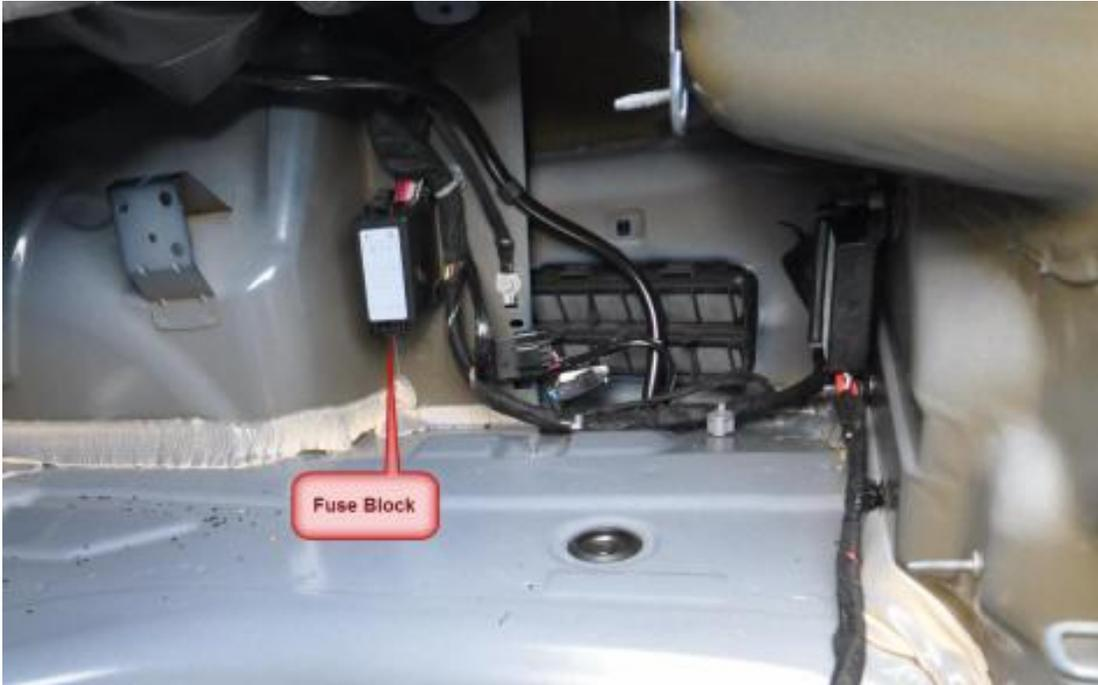
Caution: All fuse location in rear of the Camaro are continuously "hot". They are not switched with the ignition. Take care to avoid shorting any connections. Also, see below for a Zero Current Drain installation. Install fuse taps at these locations with lead wires oriented down and fuses on fuse taps oriented left.
