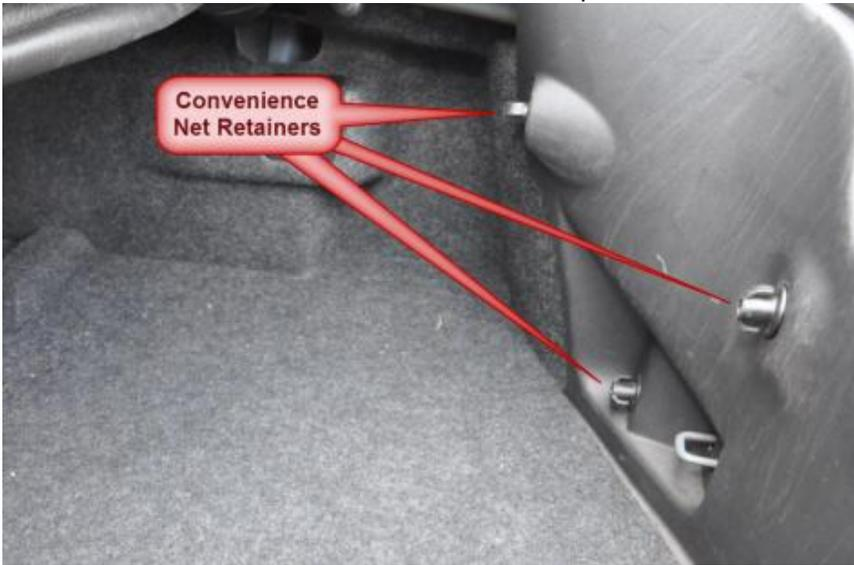
Remove black plastic threaded fastener at bottom of panel and one or two button type rivets at the top.
