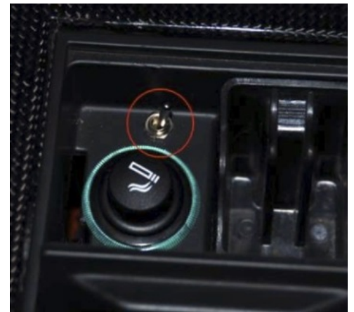
Miniature Toggle Switch mounted in ash tray
