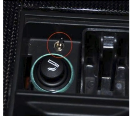
Miniature Toggle Switch mounted in ash tray
