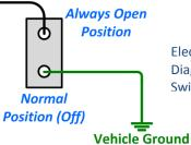
Electrical Wiring Diagram for SPST Switch
