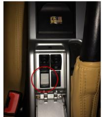
The NKK switch (above) is an exact fit for panel switch cut-outs in the Ferrari 360 and F430. E.g., NKK switch installed in the center console of a 360 Modena
