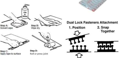
pressure to stick the mating piece in place on the mounting surface. This will assure proper alignment of the two Dual Lock pieces. Once positioned, you can take the controller off and then press the piece on the mounting surface in place to assure a firm hold.
