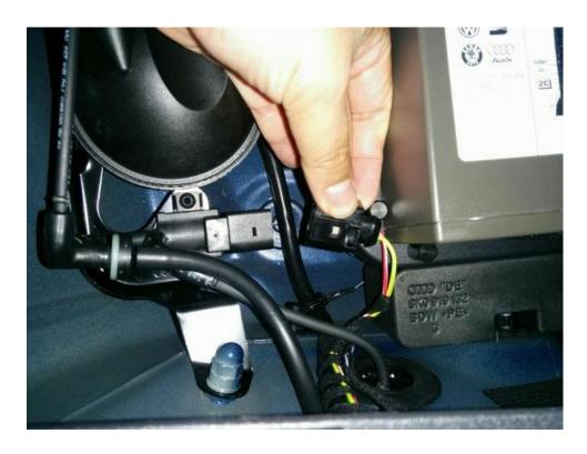
Once you have located the solenoid valve and connector, determine which of these two connectors you have ...
