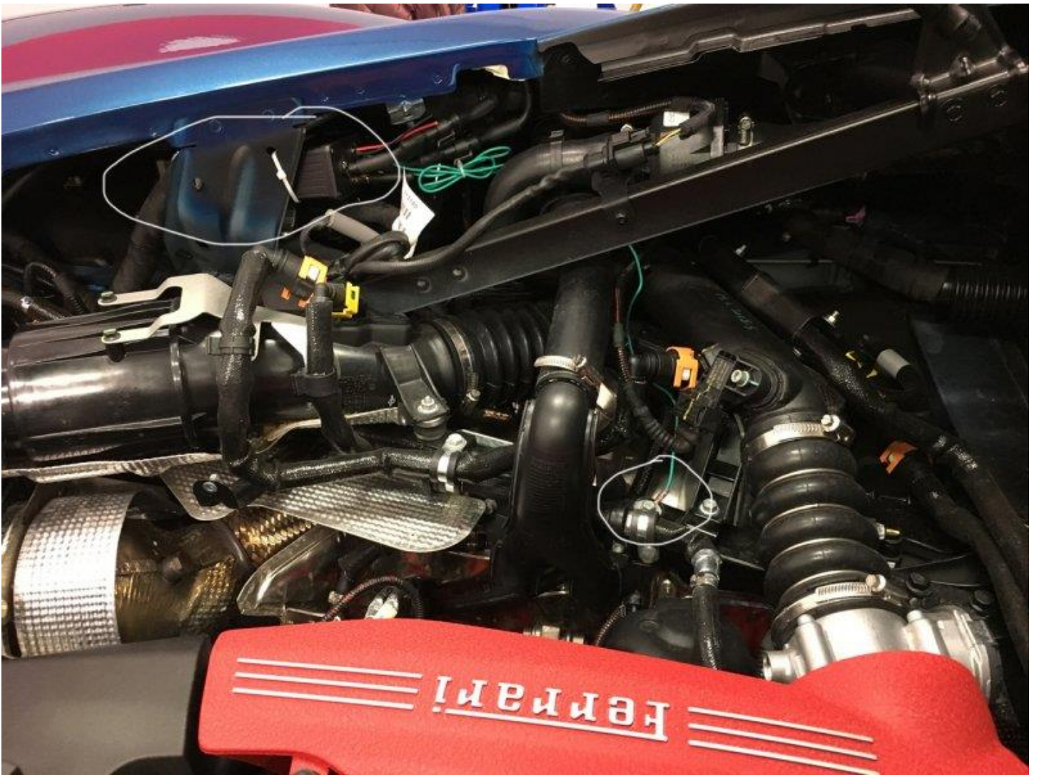
Another picture top down of the ground wire attached to the chassis:
