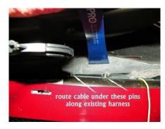
Note: You will need to provide additional wire to route power from the fuse block to the rear of the car. We recommend 18AWG or 16AWG stranded wire that is designated for automotive use. Splice into the wire provided with the controller kit. You will need approximately 10 feet of additional wire.
