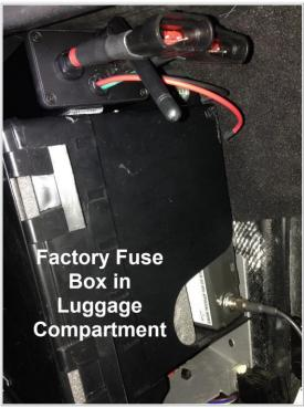
Finding a good ground point in the luggage compartment well might be a challenge as it is likely made of carbon fiber. Look for a screw or other connection point on the aluminum chassis. You should be able to find a good ground with a bit of looking. Connect the Forza Y-Cable to the adapter plugs and reinstall everything that you removed to get access.
