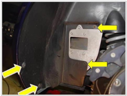
Pull back the liner to access the vacuum solenoid valve
