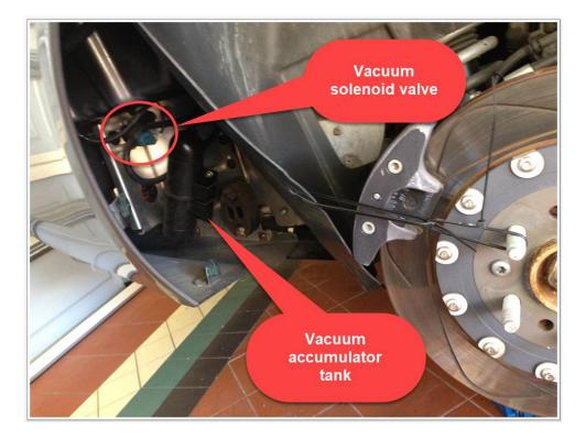
• Disconnect the existing cable from the vacuum solenoid valve.
