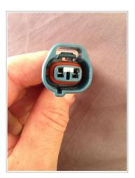
Connect adapter plugs to both the existing cable connector and the plug on the vacuum solenoid valve.
