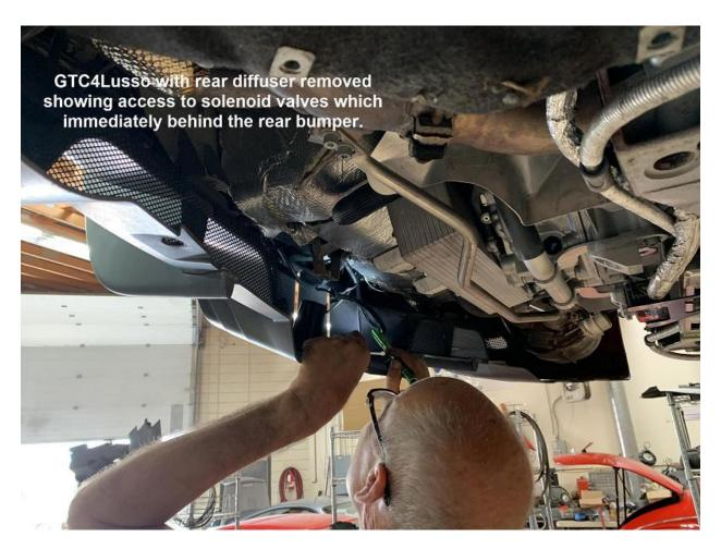
• Disconnect the cables that are currently connected to the vacuum solenoid valves. Connect the two Forza Y-Cables to the vacuum solenoid valves and to
