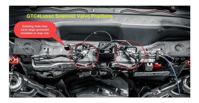
• Once the rear diffuser is removed, you will have access to reach up and behind the rear bumper to access the vacuum solenoid valves.
