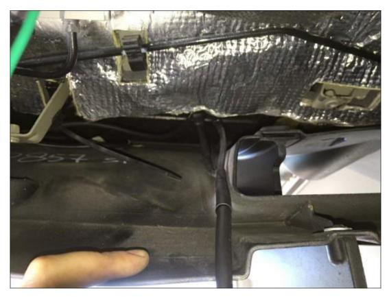
• Unplug the connector going to each solenoid and plug into the Forza cable harness. Plug the other connector of the cable harness into the solenoids.
