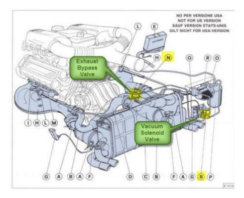
Solenoid valve for the exhaust bypass valve is located lower right area behind engine. In this photo, the vacuum tank is on the left. There is a blue plug clearly visible. There is a black plug to the right of the blue plug. The black plug which is closest to the transmission (partially hidden by vacuum lines and electrical wire) is the connecter for the exhaust bypass valve. Not the blue plug.
