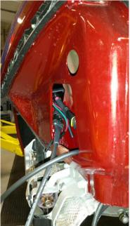
A more secure location is to route the route the cables inside the vehicle's luggage compartment and install the controller in the luggage compartment. This will require finding a suitable hole where you can pass the cable through into the luggage compartment. If a suitable cannot be found, a hole will need to be cut.
