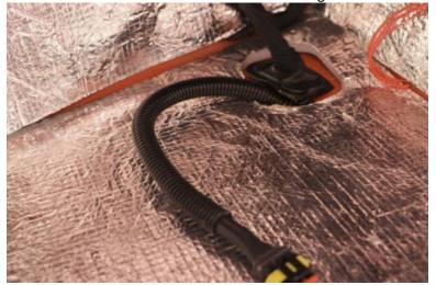
10. Mount the Forza Exhaust Bypass Valve Control using the supplied 3M Dual Lock tape. Terminate the earth cable. In this photo, one of F1 Gearbox TCU bracket bolts was used, but any suitable ground point can be used.
