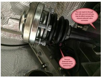
The vacuum solenoid valve is located on left side of vehicle above the gear box. The following photos were taken with the gear box removed and looking up at the left of the vehicle.
