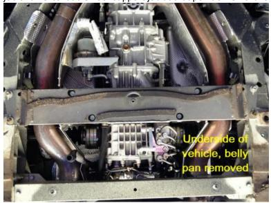
5. Once you have removed the belly pan, you can see the vacuum solenoid. This is reachable by hand. The factory exhaust solenoid is above the left half shaft, mounted to the chassis on the left-hand side of the vehicle above and to the left of the gearbox.
