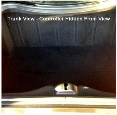
15. Refit the trunk floors. Install the belly pan underneath **REMEMBER** to connect the breather hose first. Again a 2 man job or requires an adjustable floor support tool to hold the belly pan up.
