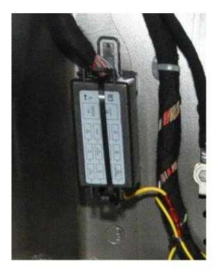
Secure the loose wires with cable ties ... Note: This photo shows the Model D1 controller. Installation of the Model E2 or B6 is similar.
