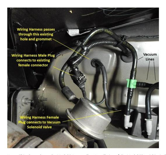
Note: This photo shows the Model D1 controller. Installation of the Model E2 or B6 is similar.
