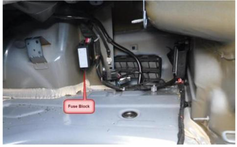
Caution: All fuse location in rear of the Camaro are continuously "hot". They are not switched with the ignition. Take care to avoid shorting any connections. Also, see below for a Zero Current Drain installation.
