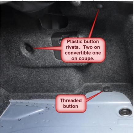
Pull back carpeted panel on right to gain access to the fuse block. Remove the fuse block cover.
