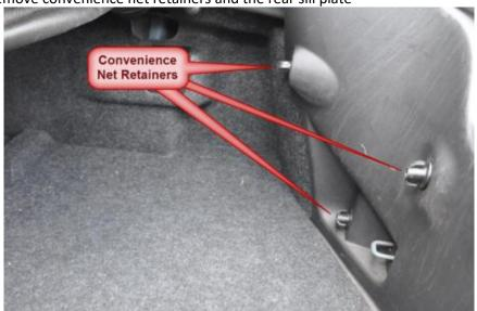
Remove black plastic threaded fastener at bottom of panel and one or two button type rivets at the top.
