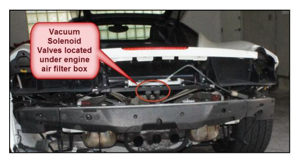
Here is a close up view of the vacuum solenoid valves ...
