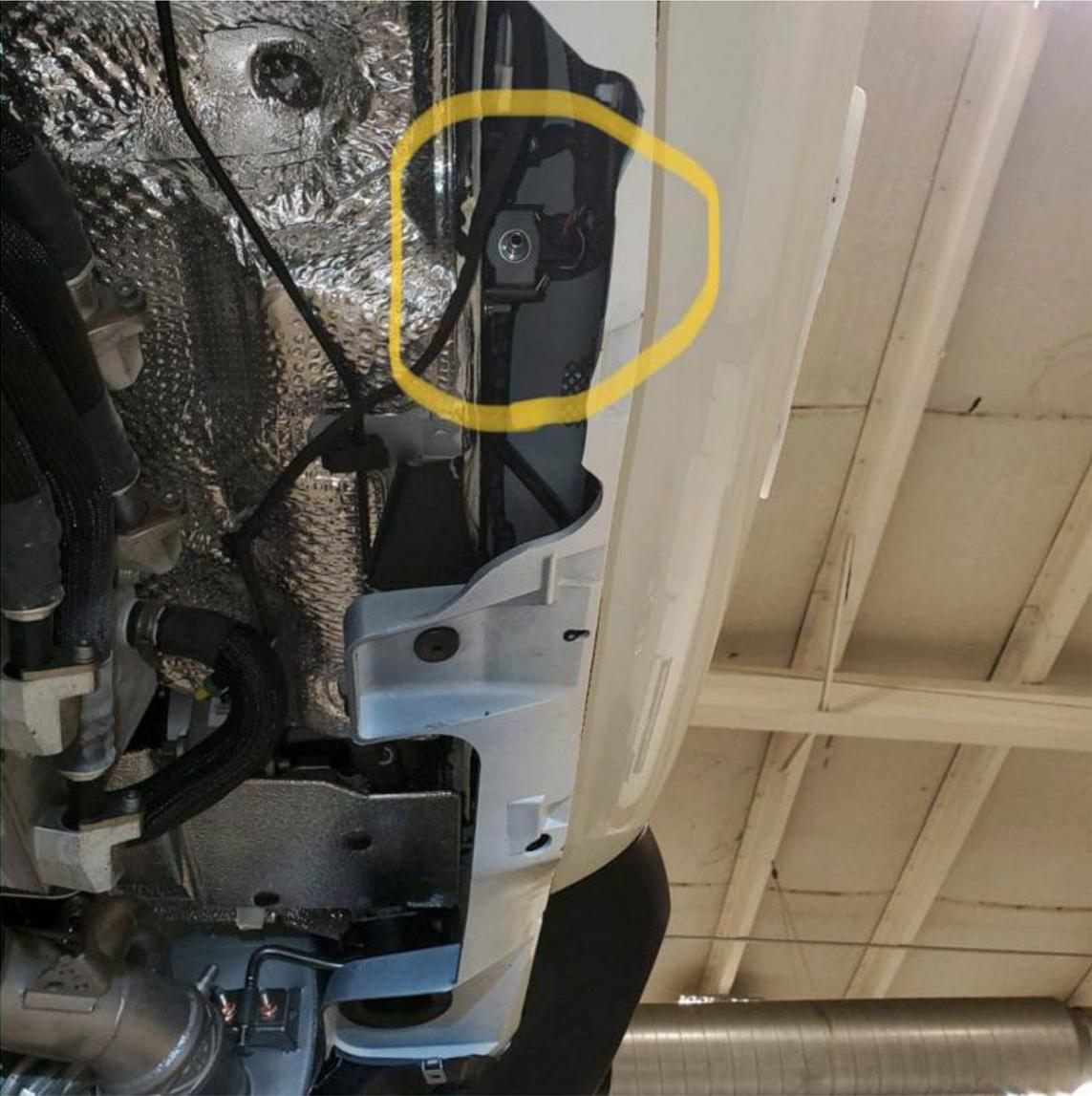
4. Find the factory grommet that leads to the car's trunk (boot). Trim some of the fabric tape off the rubber grommet and cut a small slice in the boot of the grommet to make some room to feed the cables into the trunk (boot) of the car.
