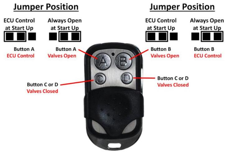
Start the engine and check operation of the bypass valves. If valves do not open when you use the remote or the manual switch, proceed with Troubleshooting on the page 6.
