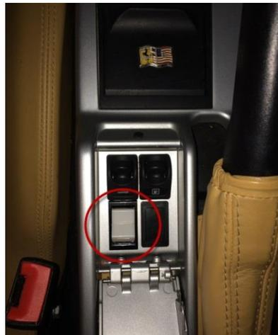
The NKK switch (below) is an exact fit for panel switch cut-outs in many Ferrari's. Here is the NKK switch installed in the center console of a 360 Modena
